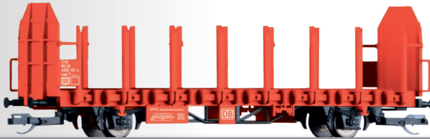
Rungenwagen Laaps der DB AG Stake car Laaps of the DB AG
