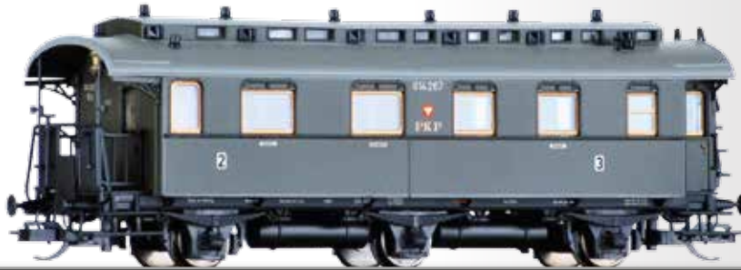
Reisezugwagen 2./3. Klasse BCiy der PKP 2nd/3rd class passenger coach BCiy of the PKP
