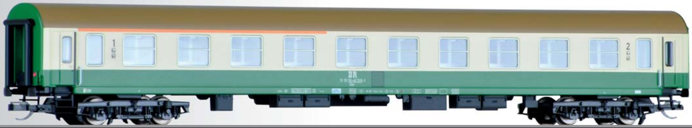
Reisezugwagen 1./2. Klasse ABm, Bauart Halberstadt, der DR 1st / 2nd class passenger coach ABm, type Halberstadt, of the DR
