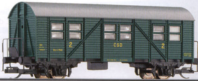
Behelfspersonenwagen Biz (ex MCI) der ČSD 2nd class passenger coach Biz (ex MCI) of the ČSD
