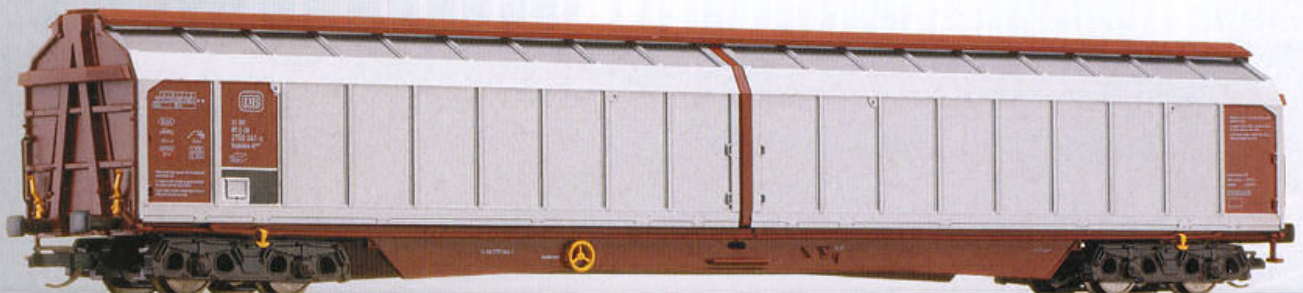
Schiebewandwagen Habbis 346 der DB Sliding cover box car Habbis 346 of the DB
