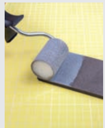
Once the glue has dried, NOCH Structured Road Construction Paint (e.g. ref. 60825) is applied.
