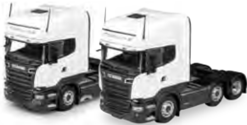
80465091, 80465092 Scania R TL 4x2 Zugmaschine / Scania R TL 4x2 rigid tractor Scania R TL 6x2 Zugmaschine / Scania R TL 6x2 rigid tractor
