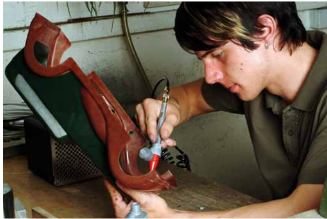
Ausbesserungen von Lackschäden aller Art. For reparations of defects in paint work.
