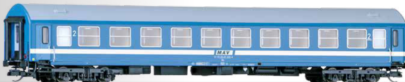
Reisezugwagen 2. Klasse Ba, Typ Y/B 70, der MAV 2nd class passenger coach Ba, type Y/B 70, of the MAV
