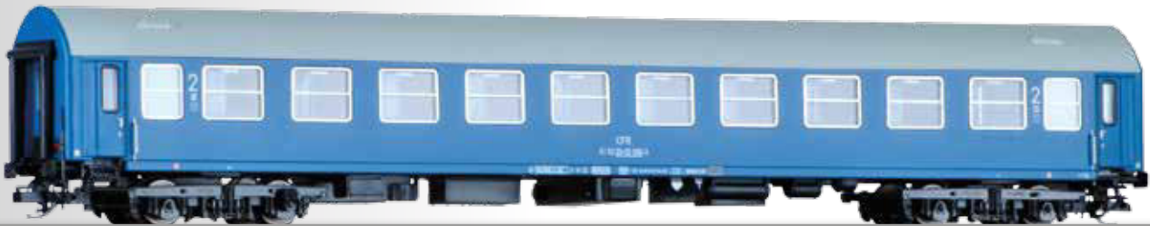
Reisezugwagen 2. Klasse, Typ Y/B 70, der CFR 2nd class passenger coach, type Y/B 70, of the CFR
