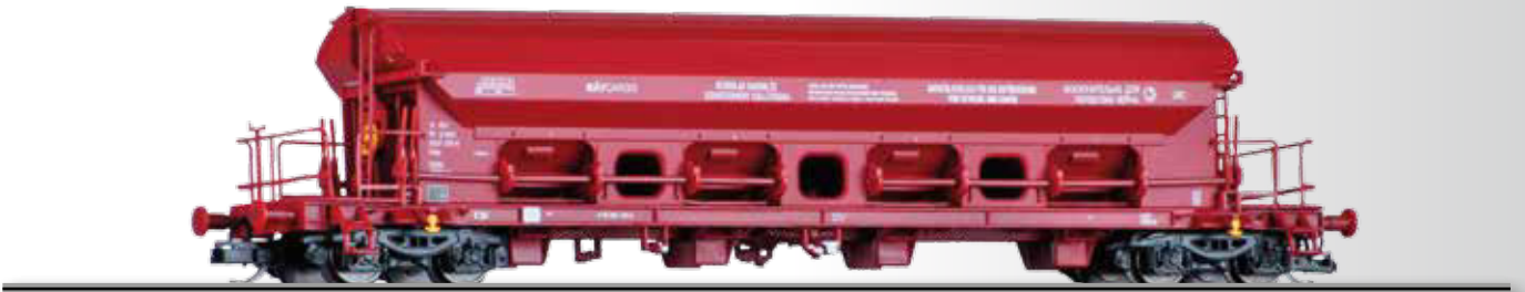
Schwenkdachwagen Tadgs der MAV CARGO Swing roof car Tadgs of the MAV CARGO
