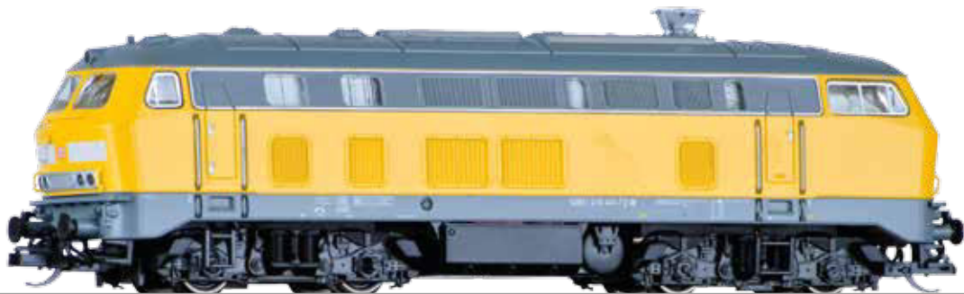
Diesellokomotive BR 218 der DB AG Diesel locomotive class 218 of the DB AG
