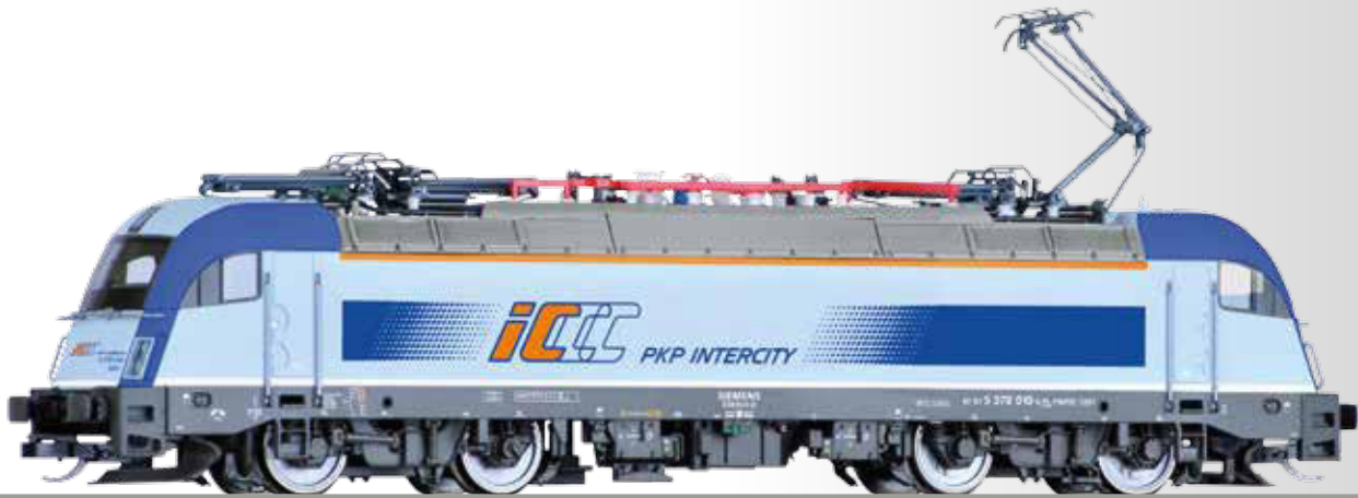
Elektr.lokomotive Reihe 370 der PKP Intercity Electric locomotive class 370 of the PKP Intercity
