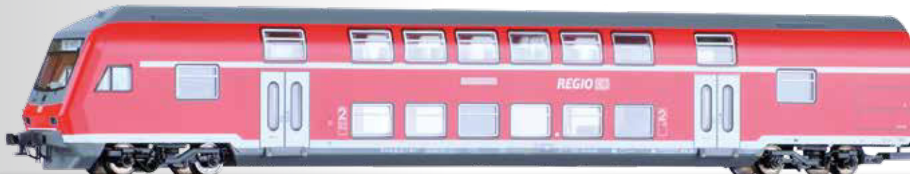
Doppelstock-Steuerwagen DBbzf 761.2 der DB AG Double-deck driving cab coach DBbzf 761.2 of the DB AG
