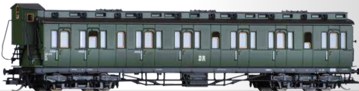
2nd class passenger coach of the DR • Mit Bremserhaus / With brakeman's cabin
