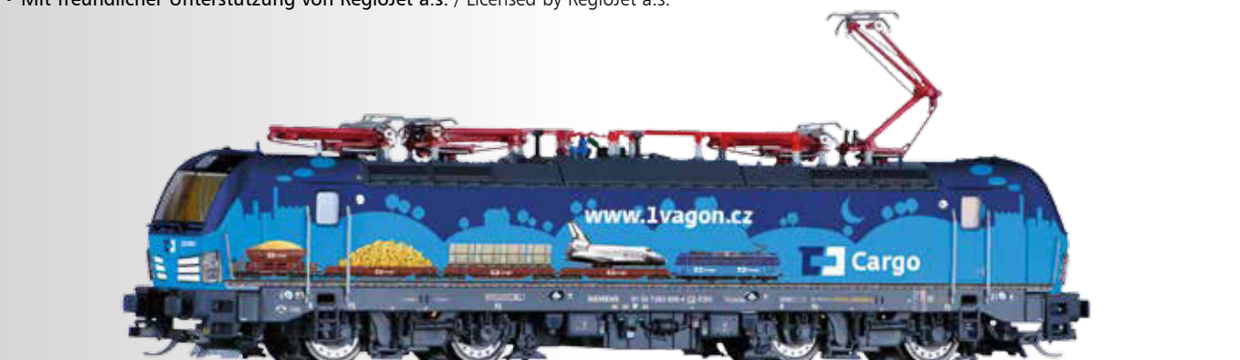
Elektrolokomotive Reihe 383 der ČD Cargo Electric locomotive class 383 of the ČD Cargo
