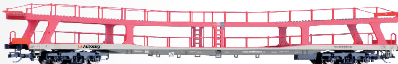
Autotransportwagen DDm 916 der DB Autozug car DDm 916 for automobile transport of the DB Autozug
