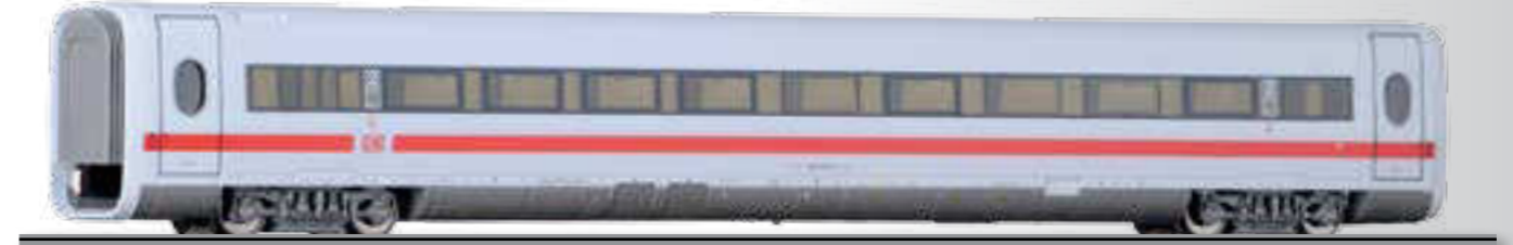
ICE 1-Ergänzungswagen 2. Klasse der DB AG 2nd class passenger coach of the DB AG, additional to ICE 1
