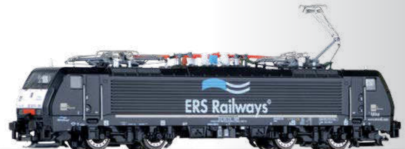
Elektrolokomotive BR 189 der MRCE, vermietet an ERS Railways Electric locomotive class 189 of the MRCE, hired to the ERS Railways
