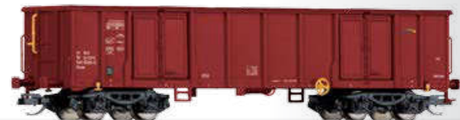
Offener Güterwagen Eaos der GYSEV Cargo Open freight var Eaos of the GYSEV Cargo
