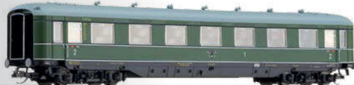
Reisezugwagen 1./2. Klasse AB4ü-39 der DRG 1st/2nd class passenger coach of the DRG
