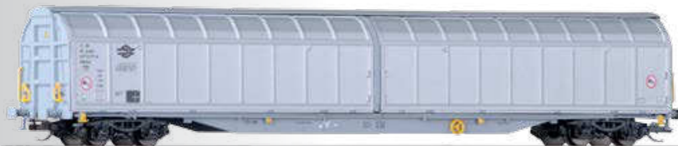
Schiebewandwagen Habbins der MAV Sliding wall box car Habbins of the MAV
