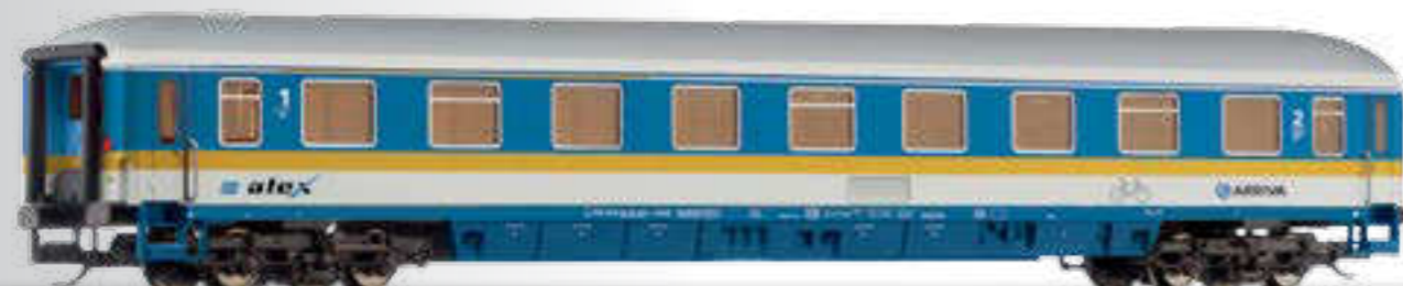
Reisezugwagen 1./2. Klasse, ABvmdz, „alex“ der ARRIVA 1st/2nd class passenger coach Abvmdz „alex“ of the ARRIVA
